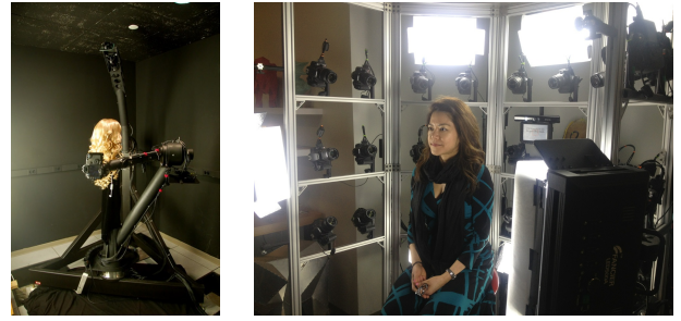
Figure 12: We use a robotic gantry to position an SLR camera at 50 views to capture the images for the wigs (left). For real hairstyles, we use a camera array of 30 SLR cameras (right).
